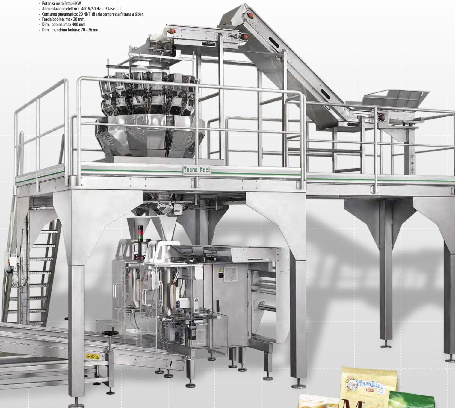
**FV 210** Vertical packaging machine mod. FV 210 (left version) electronic cantilever vertical form-fill-seal machine driven by 5 servomotors and complete with:
